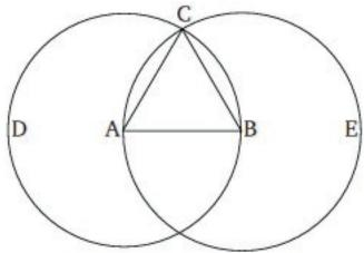
To construct an equilateral triangle on a given finite straight-line.
